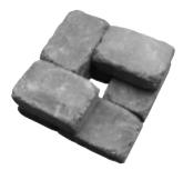
Place the second course on the first so that the joints between units are staggered from course to course and do not align vertically.
