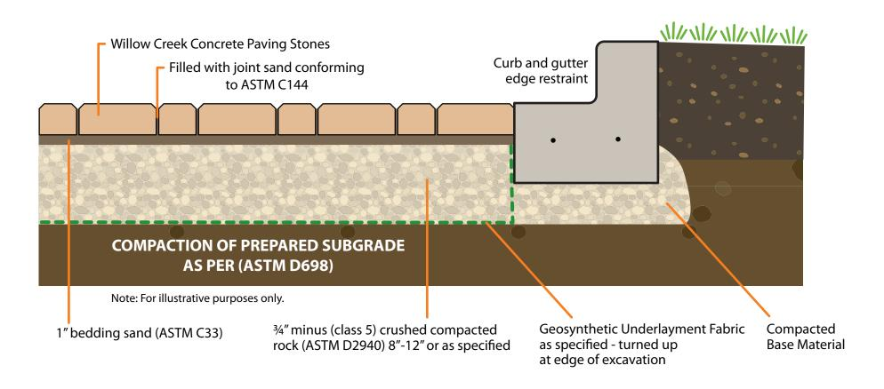
Typical Cross Section of Concrete Pavers on an Aggregate Base for Vehicular and Street Parking
